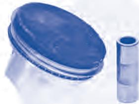
**The severe shearing forces inside Bob Teague's racing engines provide the perfect proving grounds for Dominator Synthetic Racing Oil. An entire teardown revealed virtually no bluing on the wrist pins and no piston skirt scuffing.**
