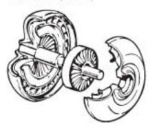
As the engine spins the impeller, ATF is forced across a small gap onto blades of the turbine, causing it to spin as well. The rotating turbine eventually provides power to the drive wheels.
