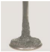
Intake valve before PI treatment.
