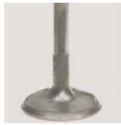
Intake valve after PI treatment.
