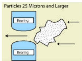
**Medium particles** are particles measuring  $25\mu$  to  $1/2"$ . While they are of greater concern than large particles because they are more difficult to remove, the threat they pose is diminished since they are still larger than many of the clearances within an engine. Their size will not allow them to enter the contact areas between many components to promote accelerated wear.
