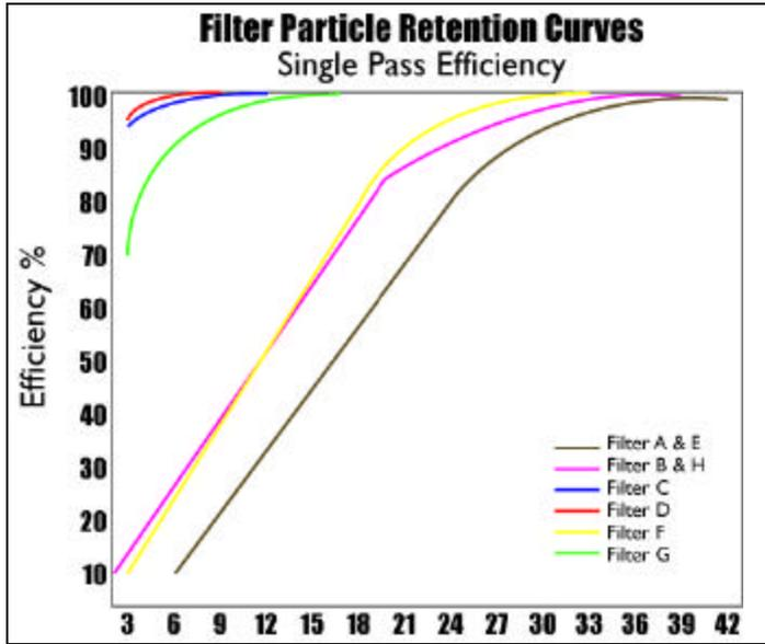
Rates charts demonstrate the correlation between superior filtration and reduced engine wear. The filters that provided superior efficiency also provided superior engine protection.
