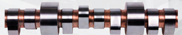
The camshaft shows little-to-no scoring, bluing or wear after 3,000 miles of high-performance racing.
