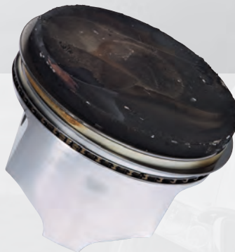
The piston crown contains normal carbon, while the rings remain clean and functional. Note the absence of wear or scuffing on the piston skirt.
