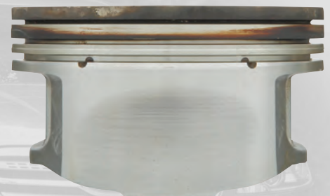
Piston After Double-Length Sequence IIIG Engine Test
