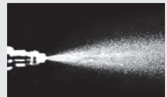
Injector spray pattern after P.i. treatment.
