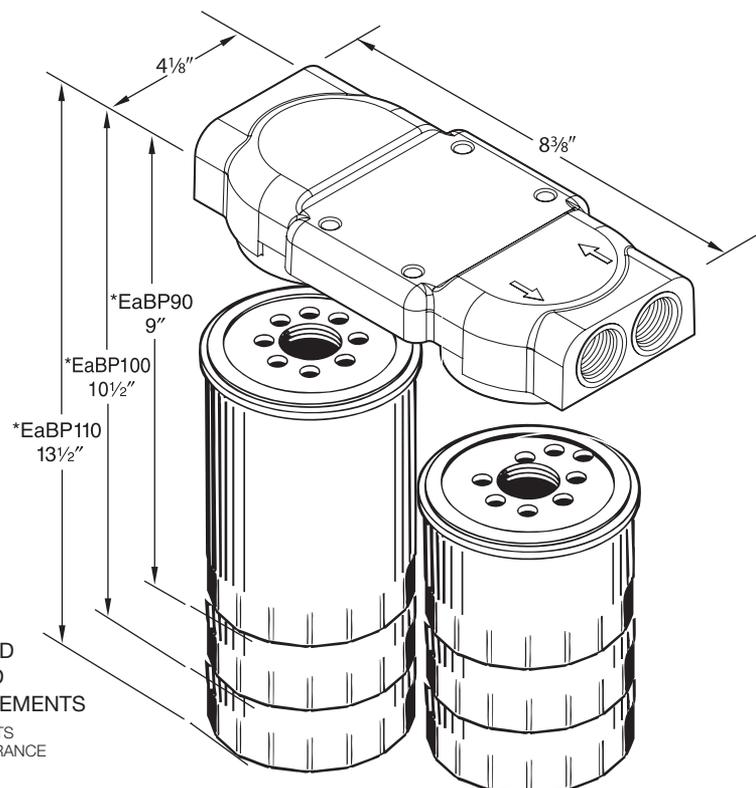
MINIMUM AREA NEEDED FOR DUAL MOUNT AND SPIN-ON OIL FILTER ELEMENTS
