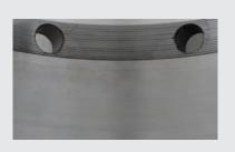
Following 512,000 miles, the transmission's output shaft bearing demonstrated no pitting or scoring despite frequent high-load operation. It earned a high wear rating of 8 out of 10, indicating only trace-light wear.
