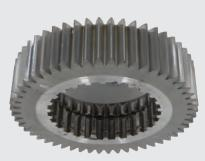
The transmission's mainshaft input drive gear demonstrated no pitting or scoring despite 512,000 miles of rigorous use. The gear earned a high wear rating of 8 out of 10, indicating only trace-light wear.
