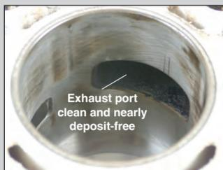
The cylinder bores demonstrated no scuffing and the cross-hatch pattern is 100% intact. The exhaust ports earned a nearly perfect rating for deposits. HP Marine delivers the protection your two-stroke engine needs.
