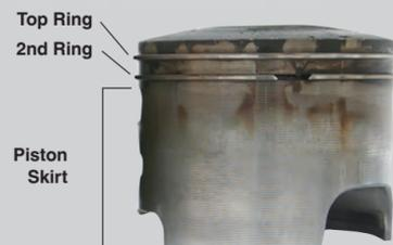
The piston rings earned a perfect merit rating, demonstrating no-stick performance. The piston skirts contained no scuffing, proving HP Marine's superior lubricity and friction-reduction capabilities.
