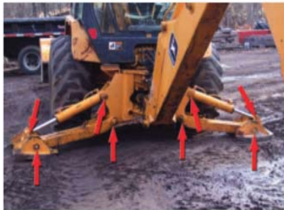
OEM recommendation: Lubricate stabilizer bearings and cylinder every 10-50 hours.
