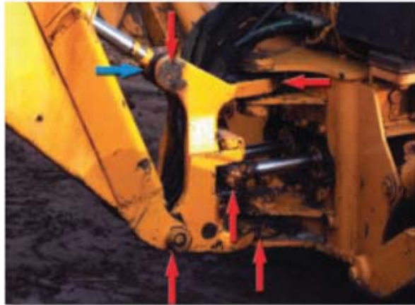
OEM recommendation: Lubricate swing frame every 10 hours.
