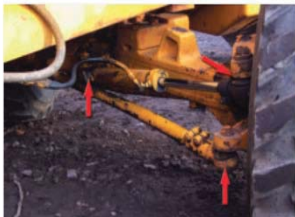
OEM recommendation: Lubricate stabilizer bearings and cylinder every 10-50 hours.
