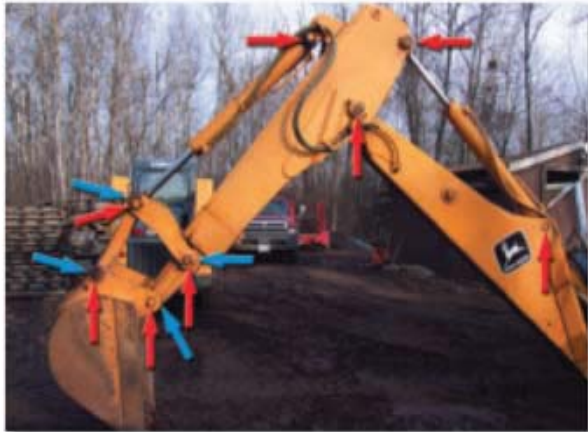
OEM recommendation: Lubricate backhoe arm, stick, bucket, cylinder bearings and linkage every 10 hours.
