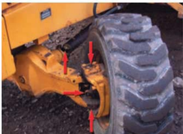
OEM recommendation: Lubricate axle universal joints and kingpin bearings every 250 hours.
