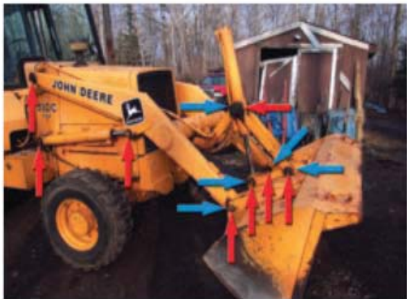
OEM recommendation: Lubricate loader bucket pivot and linkage every 10 hours.
