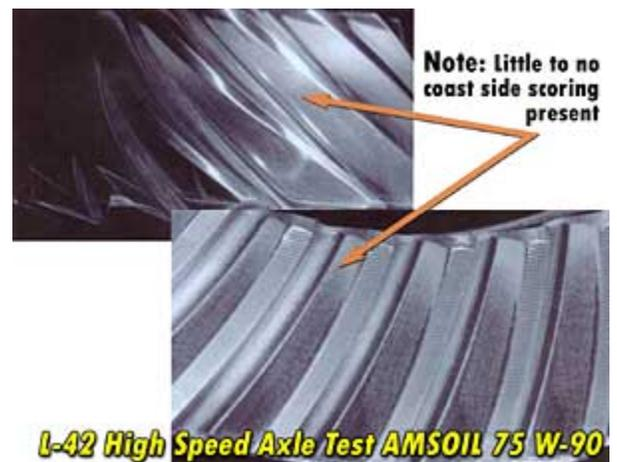
amount of scoring is evident. The same holds true for the drive gear and opinion; only the coast side is rated unless significant scoring is present, at which time the drive side is considered.
