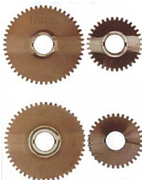
**L-60-1 Thermal Oxidation Stability Test Results**
