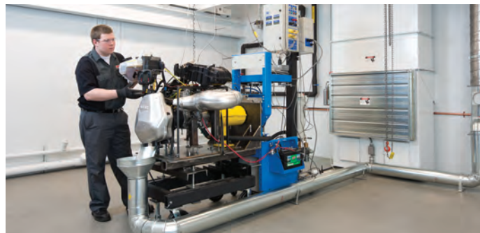
Snowmobile in-chassis testing, hand-held power equipment testing and small gasoline-engine testing will be conducted with the water brake dynamometer.
