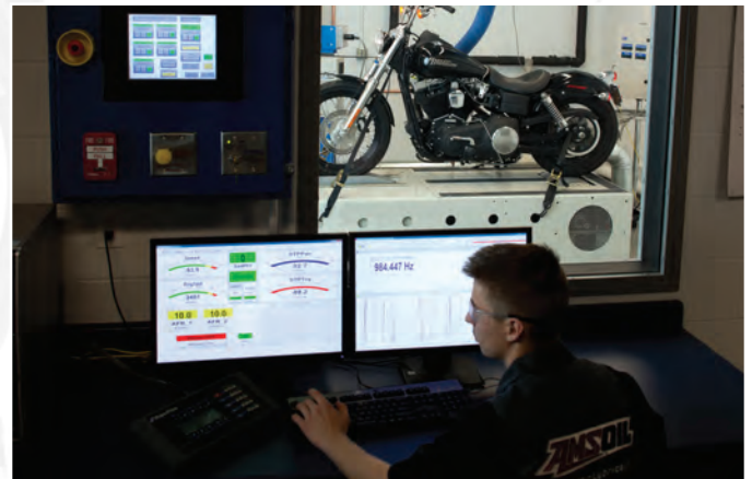
The powersports dynamometer is designed for in-chassis testing of equipment such as motorcycles and ATVs.
