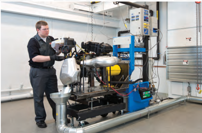
Snowmobile in-chassis testing, hand-held power equipment testing and small gasoline-engine testing will be conducted with the water brake dynamometer.
