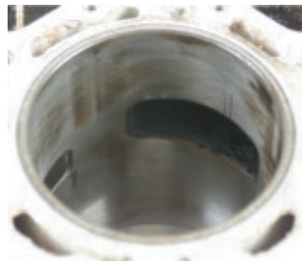
This photo shows one of the cylinders from the hp Injector-lubricated engine. Note that the original cross-hatch pattern is still visible. The scratch marks above the exhaust port are the result of a mechanical phenomenon; they appear in the exact same spot on the XD100-lubricated cylinders.
