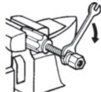
3. Screw nipple assembly into socket using wrench on nipple hex until nipple hex shoulders against socket.
