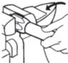
1. Place socket in vice and screw in hose counter-clockwise until hose bottoms. Back hose out ½ turn.
