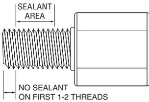
**Note:** If Teflon tape is used, it should be wrapped no more than 1½ to 2 turns in a clockwise direction when viewed from the thread end.
