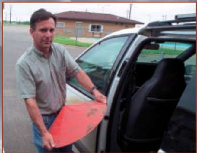
Tim Samaras holds the tornado research probe he designed. Due to its pyramid shape, wind forces it to the ground and keeps it in place as a tornado passes over.
