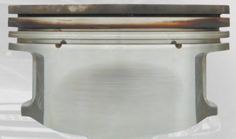
Piston After Double-Length Sequence IIIG Engine Test
