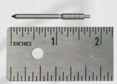
High-Pressure Common-Rail (HPCR) Fuel Injector Pintal
