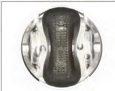
The piston undercrown is clean and free of deposits despite the extreme temperatures, demonstrating the oil's excellent detergency.
