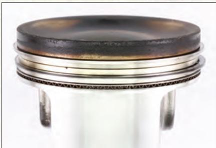
The piston is free of heavy crown deposits with no stuck rings for maximum compression and power. The skirt contains no scuffing despite severe operation at high temperatures and boost pressure.
