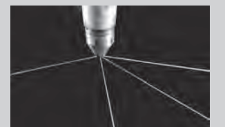
Dirty Fuel Injector Spray Pattern
