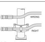
3. Protect from hazardous environment Keep hose away from hot parts. High ambient temperature will shorten hose life. If you can not route it away from the heat source, insulate it.
