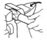
1. Place socket in vice and screw in hose counter-clockwise until hose bottoms. Back hose out 1/2 turn.
