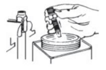
2. Oil inside of hose and the tapered nipple thread areas liberally with oil. Do not oil hose cover. Apply anti-seize to all thread areas.
