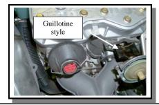
closed position, covering a portion of the exhaust port. In this position, low and lower speed performance is maximized. As the engine reaches higher operating speeds, the valve is retracted creating a larger exhaust port. The end
