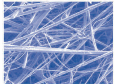
Small, consistent synthetic fibers trap smaller and hold more contaminants. Restriction is lower and flow improved.
