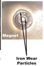
Even when vehicle manufacturers do not specify to change the factory-fill gear lube to remove wear particles, it is a good practice to do so. For optimum gear and bearing life, AMSOIL recommends the factory-fill differential gear lube be changed no later than the first 5,000 miles with new or rebuilt gears, followed by 50,000 mile drain intervals in severe service or 100,000 mile drain intervals in normal service when using AMSOIL synthetic gear lubes.
