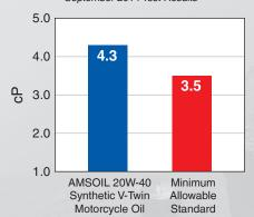
The High-Temperature/High-Shear Viscosity Test measures a lubricant's viscosity under severe high-temperature and shear conditions, similar to severe operating conditions experienced by motorcycles.
