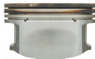
Signature Series After 200 Hours (Pass)
