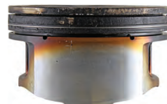
Competitor's Oil After 100 Hours (Fail)
