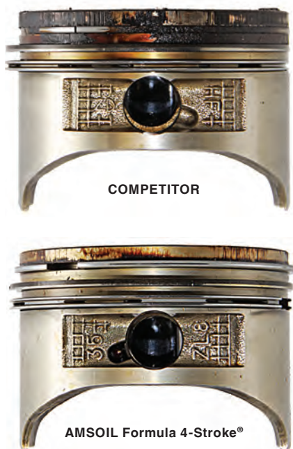
The pistons above were used in a proprietary AMSOIL severe-service four-stroke small-engine test in December 2014. The test, which runs 125 hours at 260°F, put AMSOIL Formula 4-Stroke Small Engine Oil up against a specialized competitive oil designed for commercial applications.
